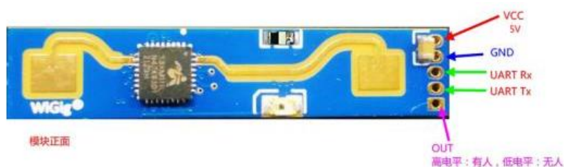
Figure 6 Module pin definition diagram
