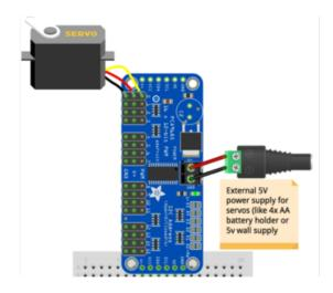
Servo orange wire to breakout PWM on channel 0 Servo red wire to breakout V+ on channel 0 Servo brown wire to breakout Gnd on channel 0 Check your servo data sheet to verify how to connect it!
