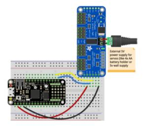
Board 3V to sensor VCC Board GND to sensor GND Board SCL to sensor SCL Board SDA to sensor SDA
