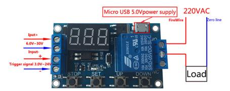
Weak control the strong electric wiring diagram
