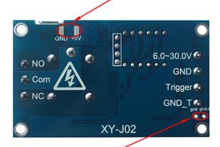
By shorting the two pads can signal GND and systems GND to link
