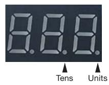
888. Decimal point in "Units" place, range: 1 second ~ 999 seconds 88.8 Decimal point in "Tens", range: 0.1 seconds ~ 99.9 seconds 8.8.8. 3 decimal points, range: 1 minute to 999 minutes
