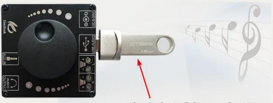
Plug in the U disk, open the APP to switch the "U disk" mode, accompanied by a prompt sound, enter the U disk playback mode.
