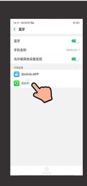
When the Bluetooth board is powered on, the blue LED flashes quickly and enters the Bluetooth connection mode; the mobile phone searches for XinYi, clicks "XinYi" to complete the connection and the sound is played, at this time the blue LED enters a long light state; open the mobile phone to play music, The blue LED flashes slowly and enters the playback state.
