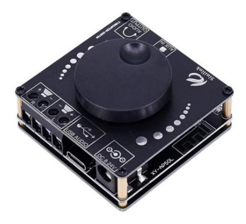
Name: 50W+50W stereo bluetooth digital power amplifier board Model:XY-AP50L
